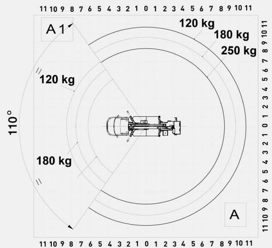
closed until boom angle 40°; Jib free with boom angle >= 40°
